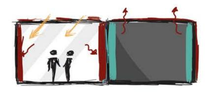
the pcm walls in the occupied space slowly warm up (by sun/electronics/people etc.), while the pcm walls in the unocciped space cool down
