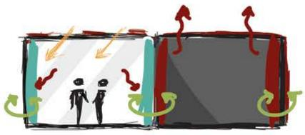
after a while the walls switch places and facilitate a stable temperature in the occupied spaces
