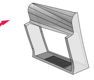
FACADE FRAME PROVIDES DOUBLE FACADE CAVITY, LINKED TO VENTILATION THROUGH FLOOR SLAB
